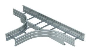
Horizontal T branch piece, for all wide span cable ladders of 160 mm side height. For further stabilisation, additional supports should be planned for the area of the fittings.
