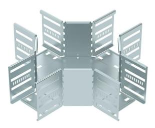
Cross-over for the creation of a horizontal branch, fitting for lock and screw-on cable trays of side height 110 mm. Screwless mounting with double clamps or screw connection with FRS truss-head screws and M6 combination nuts. Can be used in indoor areas. Fastening material must be ordered separately.
