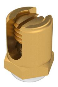
Earthing terminal for fastening the equipotential bonding wire to the cable support system. M12 threaded pin with slot. Suitable for conductor cross sections of 4-50 mm². With serrated washer and lenshead screw.
