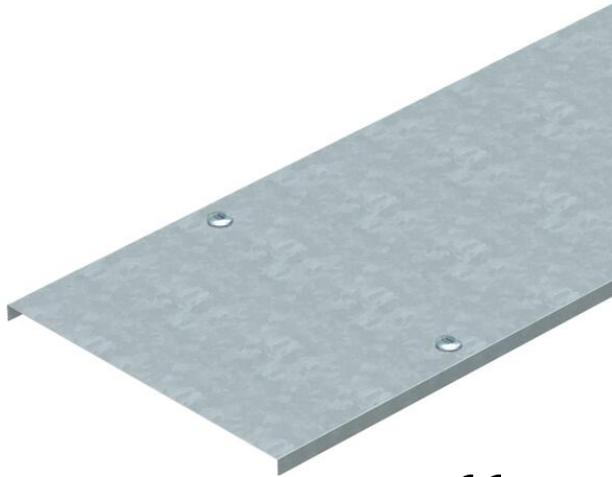
Cover for cable trays and cable ladders with three pairs of turn buckles. Transverse bead from 500 mm width. When using covers outdoors, additional measures against the influence of wind must be taken. Cover clamps or turn buckles on their own are not sufficient securing elements against wind loads.
