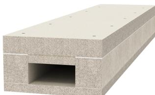
Fire protection duct made from water and frost-proof fibreglass light concrete of building material class A1 according to EN 13501-1 for fireproof laying of cables in rescue and emergency routes, and for the maintenance of electrical functionality of safety-relevant systems. Classification I120 as I duct according to DIN 4102 Part 11 and classification E90 as E duct according to DIN 4102 Part 12.
