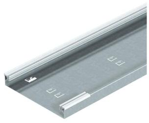
On-floor trunking base, 1 compartment, for blank/mounting lid with slope on one side, with plug-fit aluminium side profiles for layering and fixing the trunking lid, metal floor base with holding shackles for max. two plug-in, self-contacting dividers and groove for earth conductor clamp. Trunking height suitable for installation of service outlets of nominal size 2.
